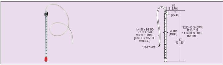
Provide visual indication of pressure with the Series 1213 Gas Pressure Manometer. Designed for use with natural gas, the manometer can also be used to monitor any compatible gases up to 15 inches of water column. Tap water is used as the sensing media and a magnetic clip provides temporary or permanent mounting. Economically priced and made of durable plastic for years of trouble-free service. Includes 3´ of vinyl tubing and 1/8´ nylon male NPT to barb fitting.
