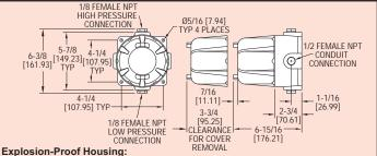
Cast iron base with aluminum cover. Rated Class I, Div. 1 & 2, Group D; Class II, Div. 1 & 2, Groups E, F, G; Class III and NEMA 7 CD, 9 EFG. Wt. 7-1/2 lbs (3.4kg). Switch must be factory installed. Change base number to 1824 and add EXPL suffix
