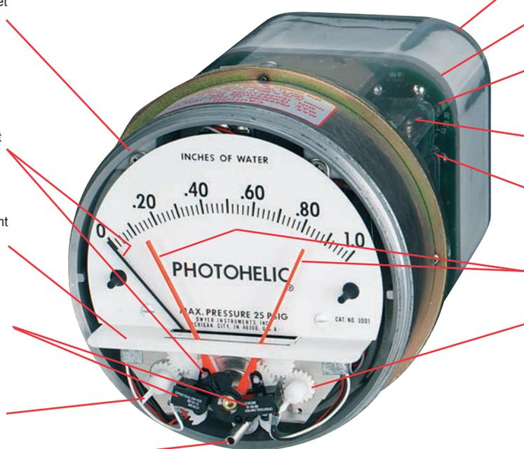
**Plastic enclosure** protects electronic components and electrical connections.
