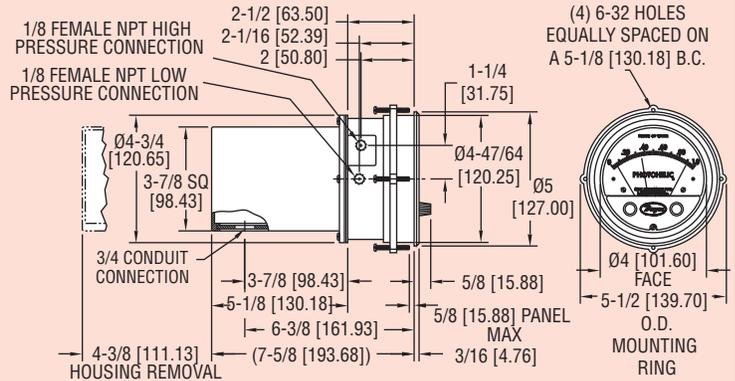
**Photohelic® Switch/Gages** function as versatile, highly repeatable pressure switches combined with a precise pressure gage employing the time-proven Magnehelic® gage design. The Photohelic® gage measures and controls positive, negative or differential pressures of air and compatible gases. Standard models are rated to 25 psig (1.7 bar) with options to 35 (2.4) or 80 (5.5 bar) psig. Single pressure 36000S models measure to 6000 psig (413 bar) with a 9000 psig (620 bar) rating.
