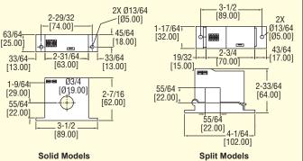
**The Series CCT60/70 True RMS Current Transformers** are a low cost alternative for providing true RMS outputs on distorted AC waveforms. True RMS outputs are ideal for nonlinear loads or noisy circuits. For existing installations, split core models can be installed without disconnecting cables. Each model offers three jumper selectable ranges to reduce the risk of ordering the wrong model.
