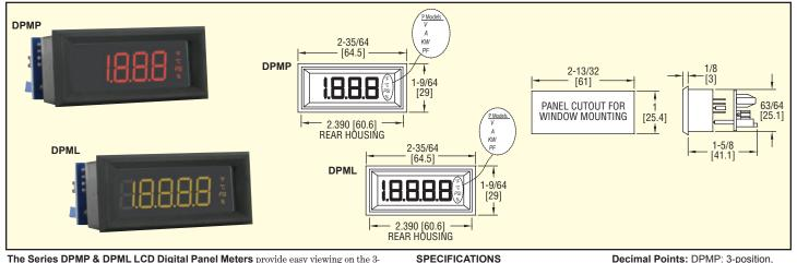
The Series DPMP & DPML LCD Digital Panel Meters provide easy viewing on the 3-1/2 or 4-1/2 digit LCD display. The display segments are available in a choice of amber, black, red or green. The meter features user-selectable engineering units, adjustable span and zero and field-selectable decimal point position. The snap-in bezel mount eliminates mounting hardware for quick installation. A 24 VDC power supply is required for the operation of the backlight.
