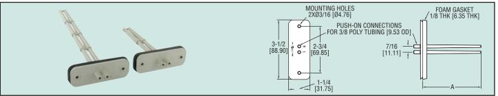
The Series PAFS-1000 Averaging Flow Sensor is ideal for sensing differential pressure in the inlet section of variable air volume terminal units and fan terminal units. Units can also be used to sense differential pressure at other locations in the main or branch duct systems.
