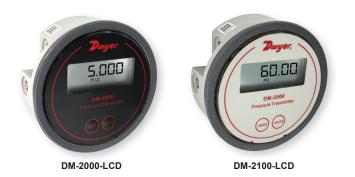
The Dwyer SERIES DM-2000 Differential Pressure Transmitter senses the pressure of air and compatible gases and sends a standard 4-20 mA output signal. The DM-2000 housing is specifically designed to mount in the same diameter cutout as a standard Magnehelic® gage. A wide range of models are available factory calibrated to specific ranges.
