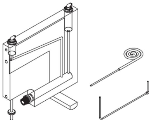
1. Remove gage from case. Set up in vertical position using (a) gage stand and leveling screw or (b) Magneclips on a vertical steel surface.
