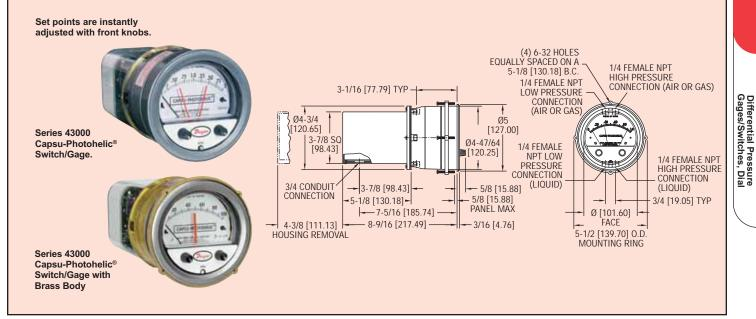
Capsu-Photohelic<sup>®</sup> Switch/Gages function as versatile, highly repeatable pressure switches combined with a precise pressure gage employing the timeproven Magnehelic<sup>®</sup> gage design. The Capsu-Photohelic<sup>®</sup> gage employs an encapsulated sensing element for use with both liquids and gases at pressures to 500 psig (34 bar). Optional cast brass case is available for water or water based liquids.
