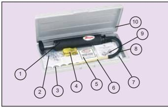
**Easy-to-Use Smoke Gage Kit** enables you to quickly balance maximum CO<sub>9</sub> with minimum smoke for clean, efficient combustion. Simply take an actual sample of the smoke being tested and compare it to the standards on the smoke chart included. Just 10 full strokes of the pump produces an accurate test sample. Complete testing instructions are included.
