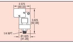
Series A1PS/A1VS Economical Pressure Switches are designed with a 15 Amp SPDT switch for direct control of pumps and motors. Available in pressure, vacuum, or compound ranges, the switches offer a field adjustable set point. Easily adjust the switch by aligning the top of the self locking adjusting nut with the desired setting indicated on the adjacent range scale. Connection is 1/4 " male NPT for quick installation and can be mounted in any position.
