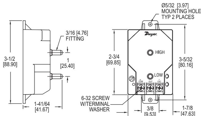
Our low cost **Series 668 Differential Pressure Transmitter** is capable of measuring low pressures with a  $\pm 1\%$  accuracy ideally suited for proper building pressurization and air flow control. Transmitters can withstand up to 10 psig overpressure with no damage to the unit. Variable capacitance sensor design provides excellent sensitivity and long-term stability. Compact, lightweight design makes installation simple and easy. Units also feature reverse-polarity protection.
