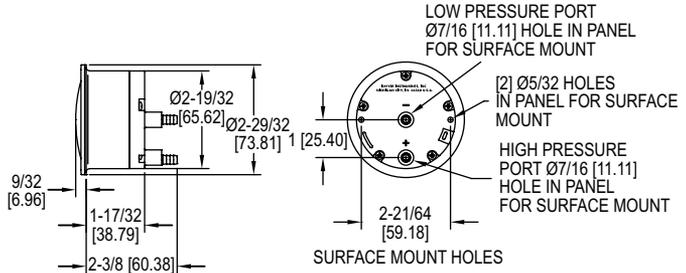
**Series 2-5000 Minihelic® II Differential Pressure Gage** has a clean design, small size, low cost and sufficient accuracy for all but the most demanding applications. With housing molded from mineral- and glass-filled nylon and a lens molded from polycarbonate, this gage will withstand rough use and exposure, as well as high total pressure up to 30 psig (2.067 bar). Over-pressure is accommodated by a blow-out membrane molded in conjunction with the diaphragm.
