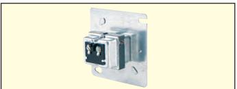
**UL** and **CSA** listed **Class 2** step down transformer is mounted on a 4-1/4" square plate stand-off for direct installation in standard 4" x 4" x 1-1/2" junction boxes. The A-699 is suitable for powering all Dwyer 4-wire transmitters and Model 660 Air Velocity Monitor.
