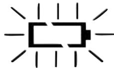
**Battery Exhausted:** Measurements are not possible. When the low battery icon indicates the battery is low, the batteries should be replaced immediately with a CR2032 lithium cell battery using the below steps.
