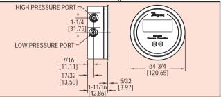
The Dwyer Series DM-2000 Differential Pressure Transmitter senses the pressure of air and compatible gases and sends a standard 4-20 mA output signal. The DM-2000 housing is specifically designed to mount in the same diameter cutout as a standard Magnehelic® gage. A wide range of models are available factory calibrated to specific ranges.
