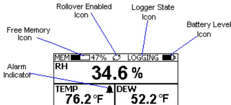
This screen shows the current Relative Humidity, Temperature and Dew Point measurements. The measurements are updated every two seconds, independent of the device sample rate.
