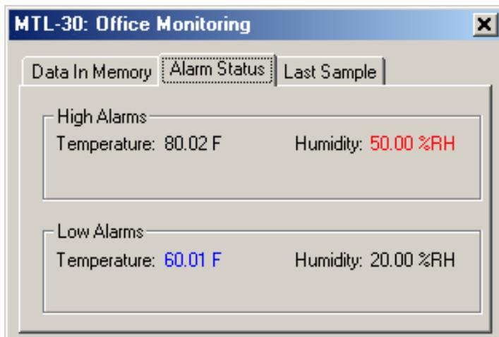
The *Alarm Status* pane displays the alarm thresholds for the active channels. If a high alarm occurred the threshold is displayed in red. If a low alarm occurred, the threshold is displayed in blue.
