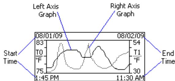
This screen shows the graph of the samples stored in logger memory. The solid line corresponds to the left axis.
