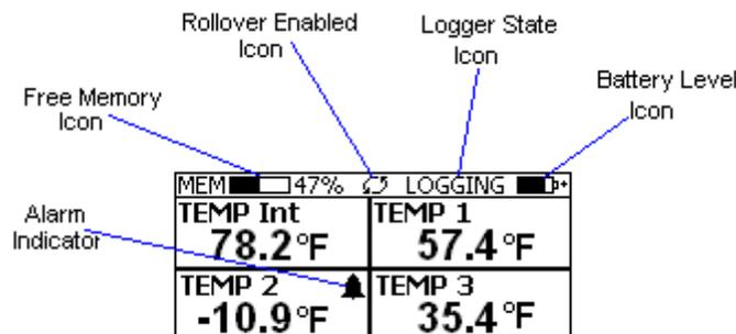
This screen shows the current temperature measurements. These measurements are updated every two seconds, independent of the device sample rate.
