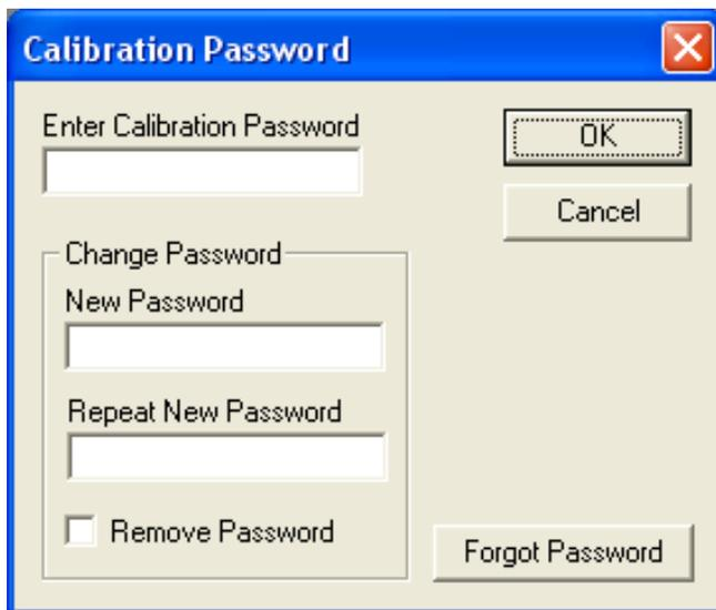
To change the calibration password select **Calibrate...** from the **Logger** menu. When the *Calibration Password* window is displayed, follow these steps:
