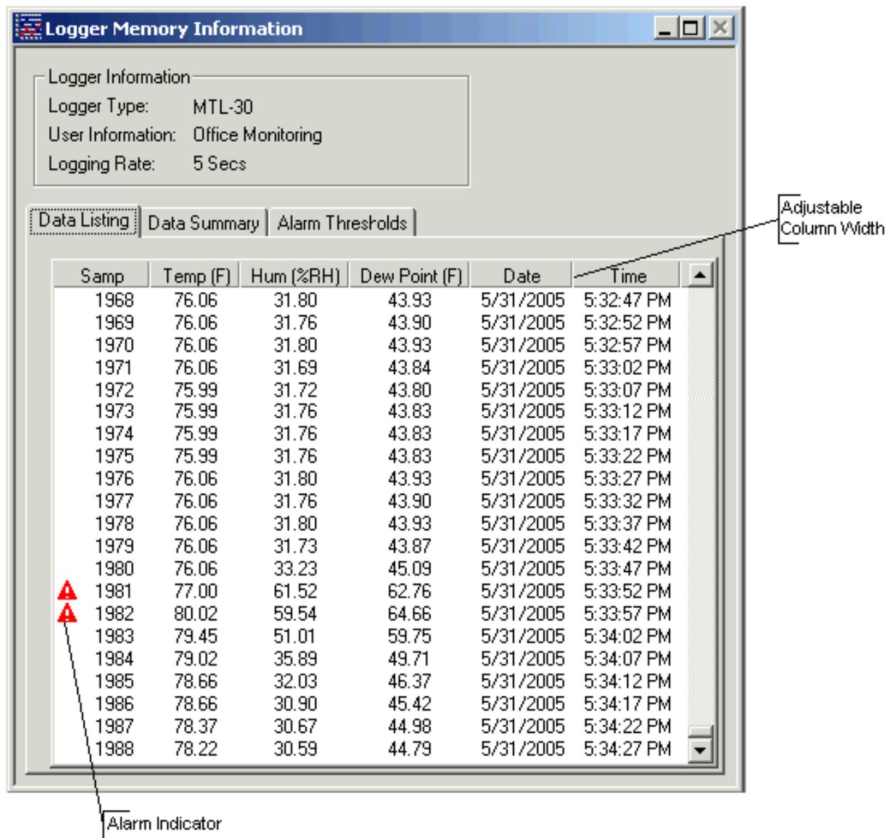
The Data pane lists the data samples collected by the logger. If the data rollover check box in the setup window was cleared, the earliest data samples are listed. If the data rollover check box was checked, the latest data samples are listed.
