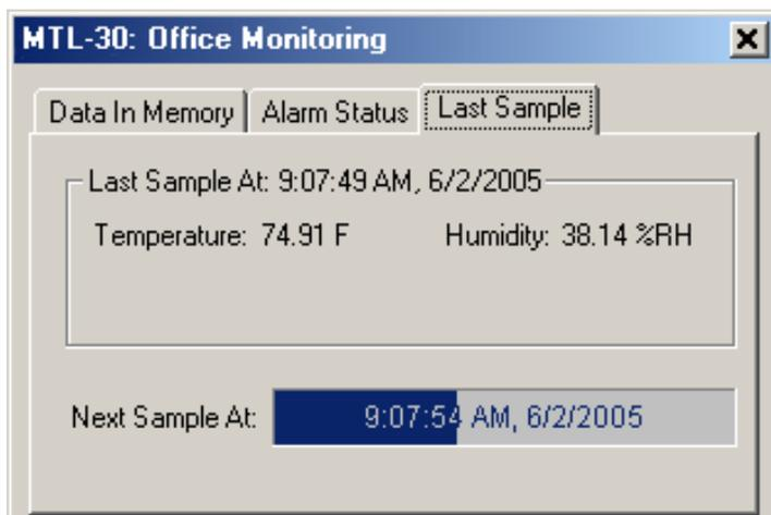
The *Last Sample* pane shows the value of the last sample taken, for all the active channels. It also shows when the next sample will be taken.
