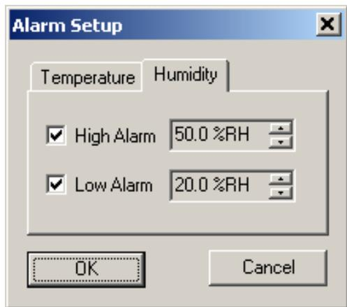
The checkbox to the left of the low/high alarms enables the alarm when checked, and disables the alarm when clear.
