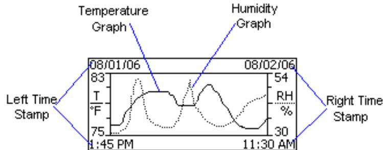
This screen shows the graph of the samples stored in logger memory. The temperature graph is shown with a solid line. The temperature axis is on the left. The humidity graph is shown with a dotted line. The humidity axis is on the right. The graph time stamps are shown on the left and on the right, above the axis.
