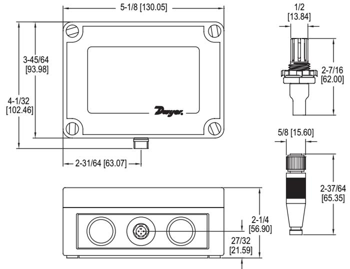
The **Series RH-R Humidity Transmitter** is the ideal transmitter for those applications where space is limited. The compact sensor is protected by a removable filter. It can be mounted up to 16 feet away from the weatherproof base. The Series RH-R is ideal for environmental chambers, rubber bladder burst detection systems and air handler applications.
