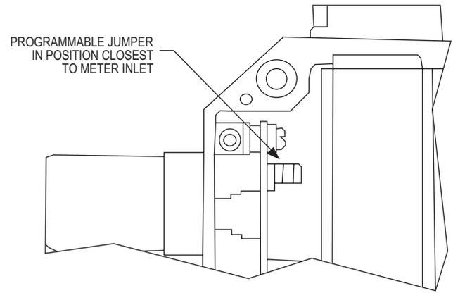
**Jumper position - 0-2000 Hz pulse out
