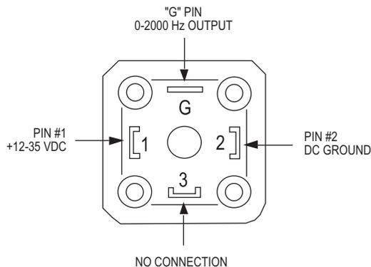
**Electrical connections - 0-2000 Hz pulse out
