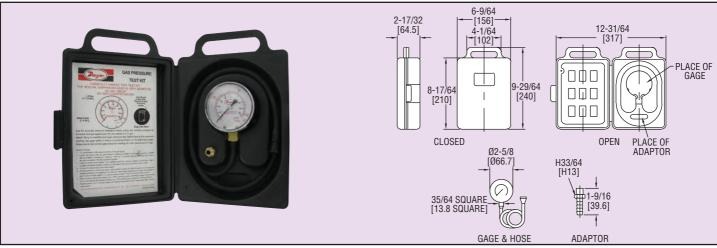
The **Model LPTK Gas Pressure Test Kit** is ideal for testing LP and natural gas lines and controls. The kit's gage shows if proper pressure is present or if a leak exists. The LPTK Gas Pressure Test Kit is available in two different gage ranges, and each gage is 3% full-scale accurate with an easy to use calibration screw on the back of the gage. It is easier to use than a manometer, and includes a sturdy case for added durability and safe handling.
