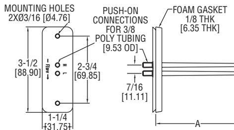
The Series PAFS-1000 Averaging Flow Sensor from Dwyer Instruments, Inc. is ideal for sensing differential pressure in the inlet section of variable air volume terminal units and fan terminal units. Units can also be used to sense differential pressure at other locations in the main or branch duct systems.
