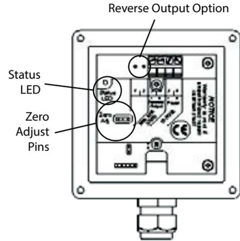
To perform the adjustment, after determining that there is a full pipe with no flow, create a short between the two pins marked "Zero Adjust". Once the red LED light comes on for approximately 50 seconds and then goes out, the zero adjustment is completed.
