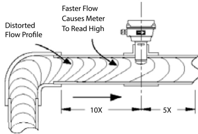
**Fitting Installation.** EFS2 Series meters require special fittings that ensure that the flow sensor is installed to the correct depth. The fitting must be installed in the pipeline before the meter can be installed. For best results, install with at least ten diameters of straight pipe upstream of the meter and five diameters downstream (or more under specific adverse circumstances). See diagrams, on page 3.
