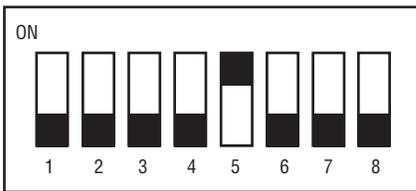
**Figure 7: Address of Transmitter is 008**
