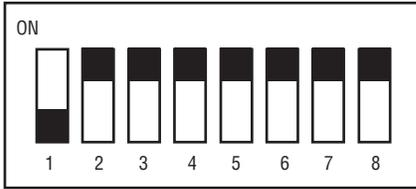
**Figure 6: Address of Transmitter is 127**
