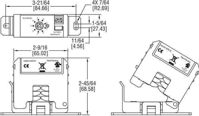
The **SERIES SSCS** Sure-Set Current Switch provides a unique approach to calibration and installing current sensors in a low cost, fast, and accurate design. Selecting the set point has never been easier, with each model having 9 pre-configured adjustable HP set points. This feature eliminates the need to work within a live enclosure, reducing the risk of arc flash on installation.
