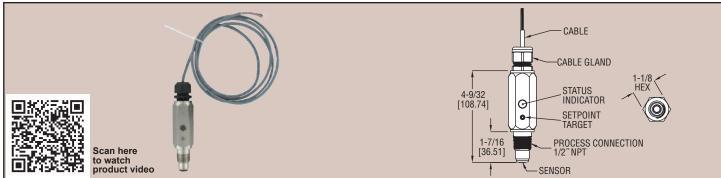
**The Series TDFS** is a thermal flow switch that indicates whether the flow rate is above or below a user set flow rate with NO and NC NPN outputs. Setpoint is easily field set, just tap the included magnet on the setpoint target three times at the desired flow rate and it's done. Incorporated into the unit are two LED status indicators on opposite sides of the unit providing visual switch indication, green when the flow is above set point, red when the flow is below set point.
