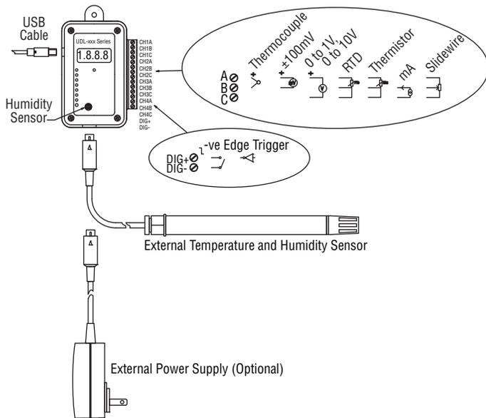
Having selected the correct sensor type, the appropriate connections can be made. The type of sensor used must be selected via the software prior to issue.
