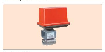
The Series BV2B incorporates a weatherproof, NEMA 4X, electric actuator powered by standard 115 VAC supply. The BV2B provides an economical weatherproof automated valve package. The modulating actuator accepts a 4 to 20 mA input for infinite valve positioning. Actuator features a single phase capacitor run motor with overload protection and a permanently lubricated gear train.
