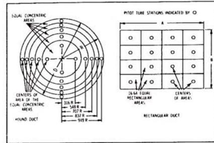
The total pressure of an air stream flowing in a duct is the sum of the static or bursting pressure exerted upon the sidewalls of the duct and the impact or velocity pressure of the moving air. Through the use of a pitot tube connected differentially to a manometer, the velocity pressure alone is indicated and the corresponding air velocity determined.
