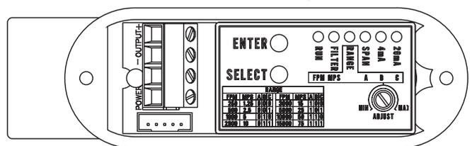
A set of controls and indicators are provided within the unit consisting of the select button, enter button, adjustment control, and six LED indicators. When operating normally, only the RUN LED indicator will be illuminated. During the setup operation the LED indicators will indicate the parameter selected, when it is being adjusted, and status of the adjustment process. If the unit is left in the setup mode for several minutes without any activity it will return to the normal operating mode.
