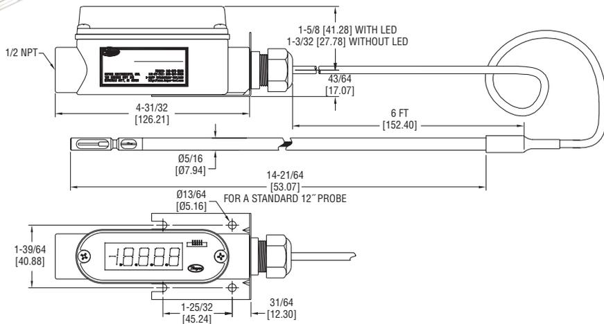
The Series 641RM Air Velocity Transmitter uses a heated mass flow sensor technology. It has 8 user selectable ranges from 250 FPM to 15000 FPM with corresponding metric ranges of 1.25 MPS to 75 MPS. The Series 641RM Air Velocity Transmitter provides an isolated 4-20 mA output proportional to the velocity. With the optional 1/2" 4-1/2 digit LED display, the Series 641RM Air Velocity Transmitter will provide a highly visible local readout of the velocity.
