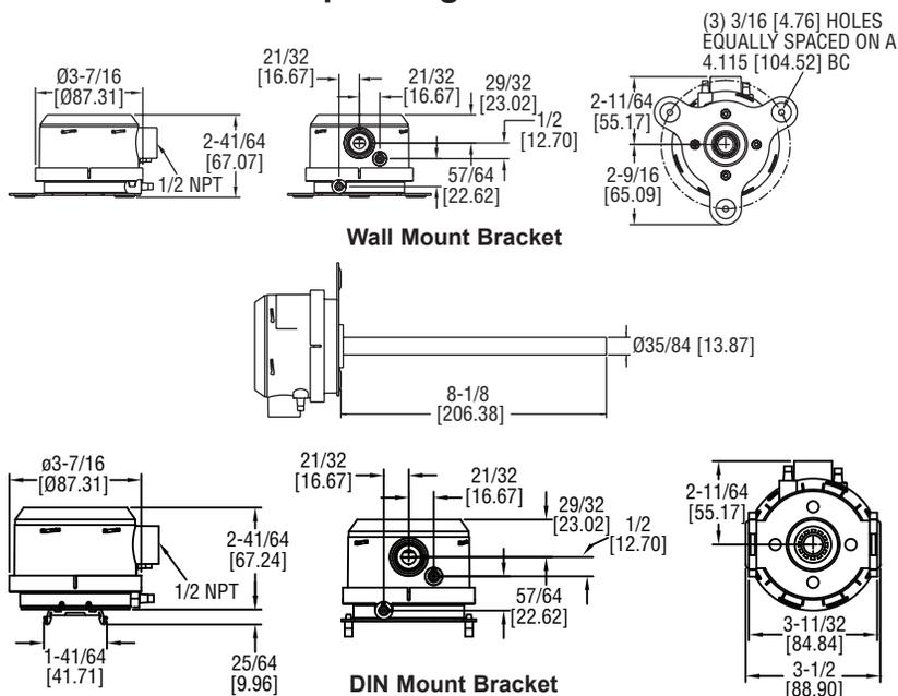
The Series MS Magnesense® Differential Pressure Transmitter is an extremely versatile transmitter for monitoring pressure and air velocity. This compact package is loaded with features such as: field selectable English or metric ranges, field upgradeable LCD display, adjustable dampening of output signal (with optional display) and the ability to select a square root output for use with pitot tubes and other similar flow sensors.
