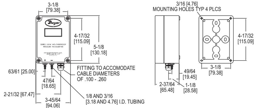
The **Series 616WL Differential Pressure Transmitter** senses the pressure of air and non-combustible, compatible gases and sends a standard 4 to 20 mA output signal. All models, including those featuring the 3 digit LCD digital read-out, are factory calibrated to specific ranges as listed in the chart below.
