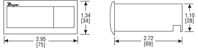
The Series TSF Thermocouple FM Approved Limit Control provides audible alarm status along with a robust 16 amp relay output. Unit allows the user to easily select automatic or manual reset along with 13 other parameters. The TSF series has a built in reset button on the front panel or can accept an external reset.
