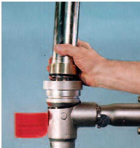
6. Slide the inner flange ring over the sight tube. When properly seated, the top of the flange ring should be flush with the bottom edge of the snap ring groove.
