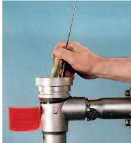
2. Place the spider over the meter tube with the "notched leg over the snorkel tube or guide rod. Slide the spider down to the meter tube's shoulder.
