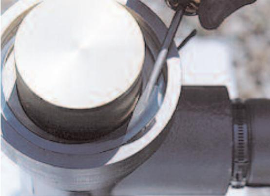
3. Using hands only, pull the sight tube straight up out of the body with a slight twisting motion, lifting it clear of the body and snorkel. The inner flange ring will lift off with the sight tube.
