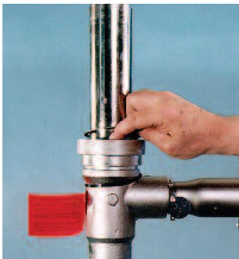
If new flow internals are used, the scale may have to be remounted on the sight tube. Depending on the model type, this can be done either by loosening the mounting screw, or reattaching the scale with double sided adhesive (new flow internals are shipped with a new scale).
