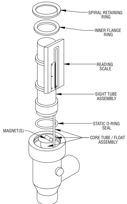
**FIGURE 2: PARTIALLY EXPLODED DRAWING OF SERIES STFLO
