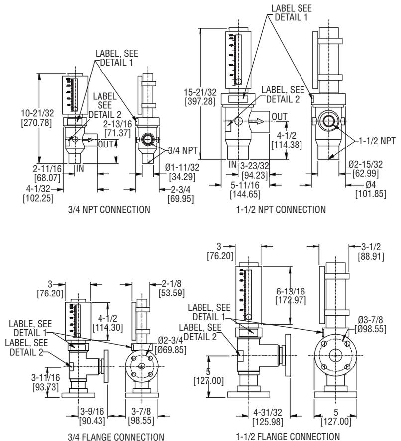
**Series STFLO Stainless Steel Flowmeters** are ideal for dirty or opaque fluids, high temperature and high pressure service and harsh environments, specifically steam applications. The direct reading scale provides  $\pm 2\%$  accuracy. Flowmeters can quickly be disassembled without removing the body from the pipeline for easy cleaning.
