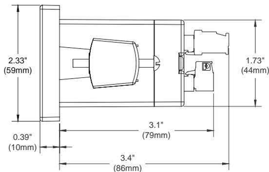
Figure 3. Case Dimensions – Top View
