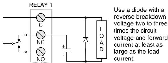
**Figure 13. Low Voltage DC Loads Protection**
