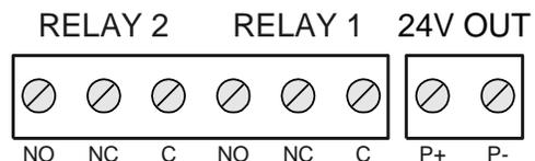
**Figure 11. Relay & 24 V Output Connections**
