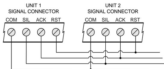
Figure 15. Shared Pushbutton Connections
