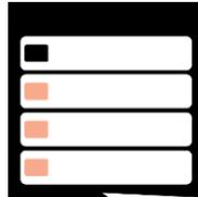
5. Press Reset to change LED 1 from off to on, setting relay 1 for fail-safe operation.
