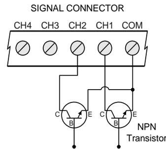
**Figure 10. Open Collector NPN Transistor Inputs**
