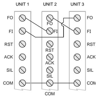
**Figure 14. System with Multiple Units Share First-Out**
