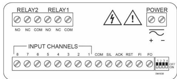
Figure 7. Connector Labeling for AN28-2
