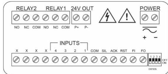
Figure 4. Connector Labeling for AN24-1
