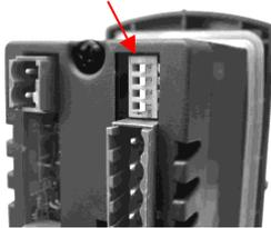
Figure 16. DIP Switch Location
