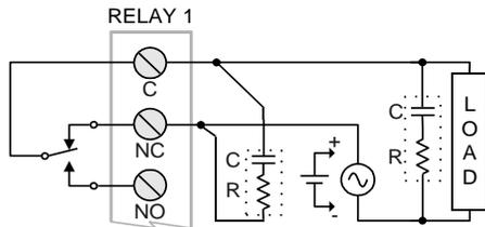
**Figure 12. AC and DC Loads Protection**
