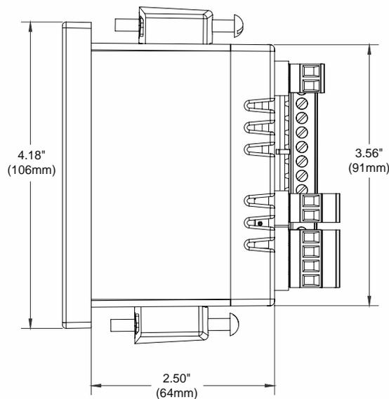
Figure 2. Case Dimensions – Side View
