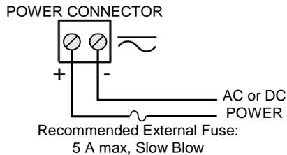
**Figure 8. Power Connections**
