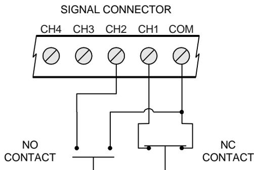
**Figure 9. NO/NC Contact Inputs**
