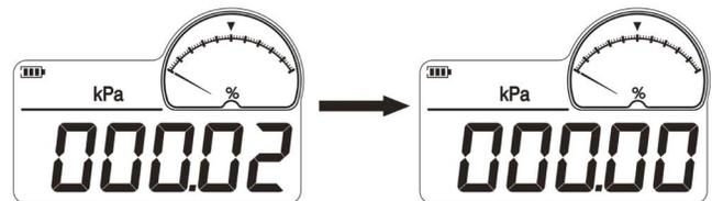
Figure 4: The Zeroing Sequence for Gage Pressure DCGII
