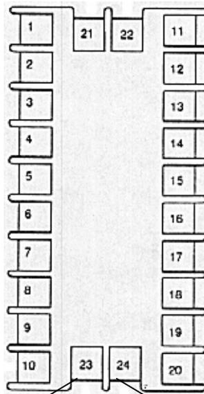
Pin 23, Signal B(+)      Pin 24, Signal A(-)
