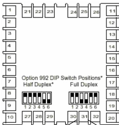
Pin 31, Signal A(-)    Pin 32, Signal B(+)
